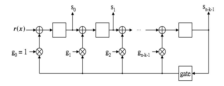
Example : Syndrome circuit for a (7,4) cyclic code with  $g(x) = 1 + x + x^3$ Received sequence r = (1001000)
