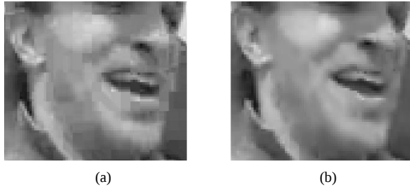
Fig. 8. Detail of the luminance output in the case of (a) loop filtering and (b) no filtering. QCIF sequence was coded at 30 kbps and 10 fps.
