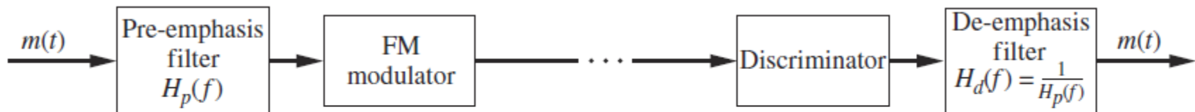
Figure 4.32 Frequency modulation system with pre-emphasis and de-emphasis.
