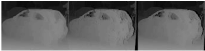
Fig. 9. Comparison between (a) reference depth map, (b) backward depth warping result, (c) backward depth warping with superpixel refinement result
