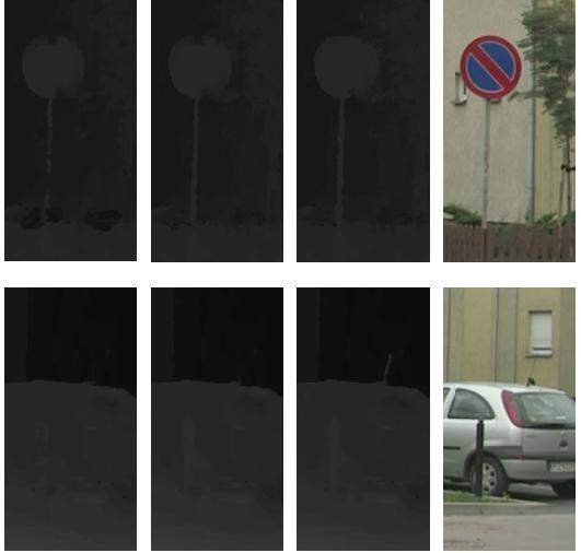
Fig. 6 Corrected depth maps and images and Post-processed depth maps: the left is  $D_{min}$ , the second is  $D_{12}$ , the third is  $D_{final}$ , and the right is  $I_{12}$
